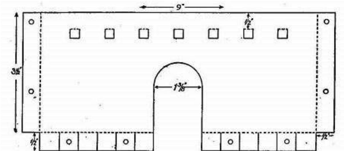
FIG. 103.—Plate for lamp chamber cut out ready for bending.
