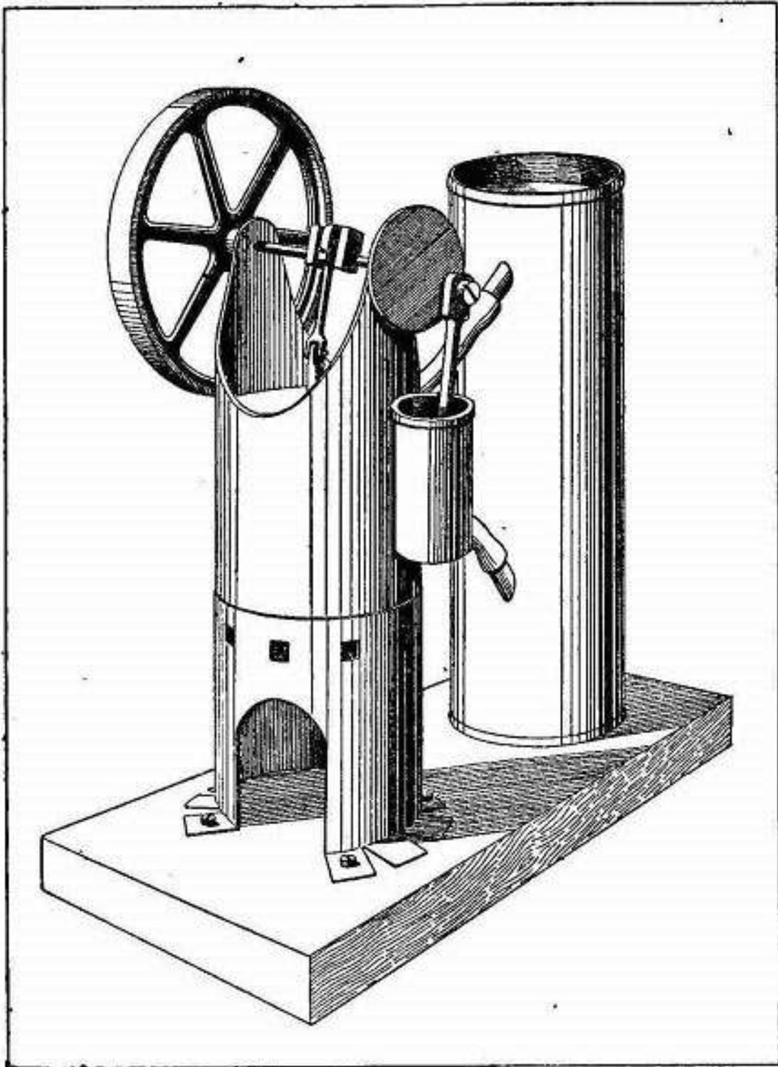
FIG. 100.—Exterior view of hot-air engine.
