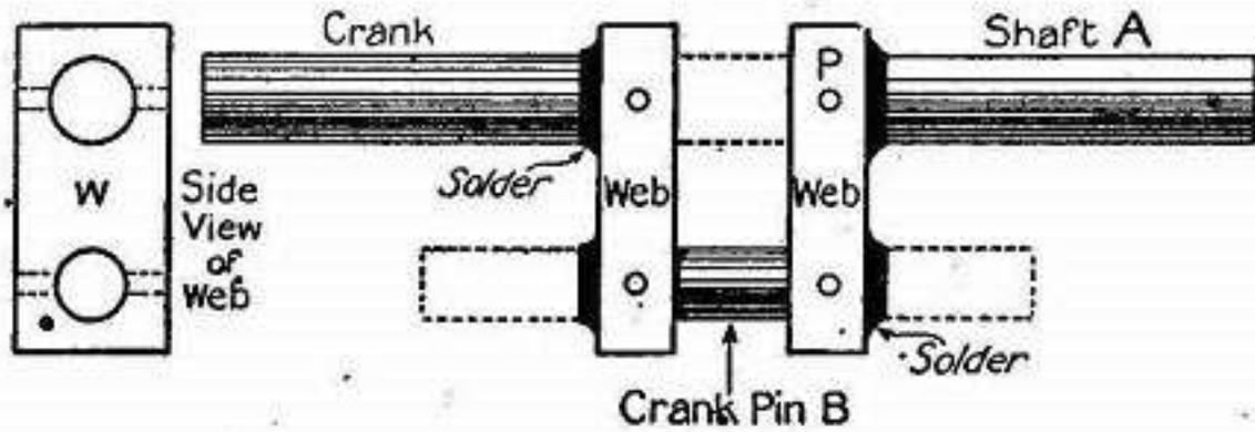
FIG. 101.—Details of built-up crank.
