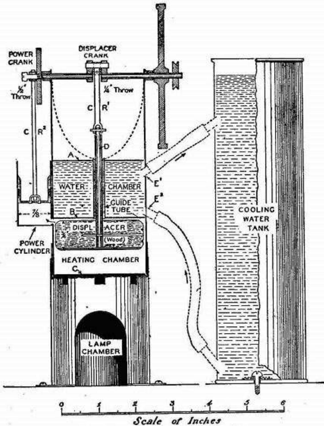
FIG. 97.—Vertical section of hot-air engine.
